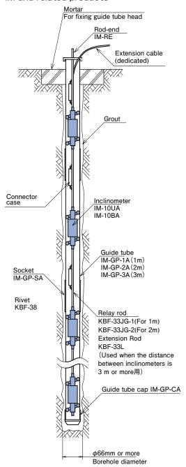
We also offer extension rods, head caps, rivets, riveters, and demountable pliers. Please contact us for details.
