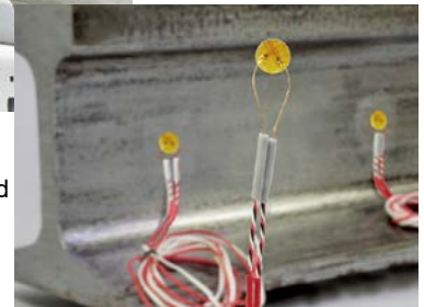
Railway axle load measurement
