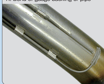
Weldable gauge AWHU and MI cable
