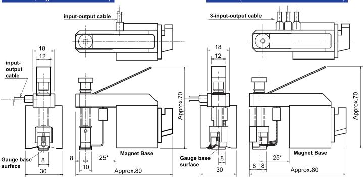
\*Dimensions when the gauge base surface is horizontal to the magnetic base. (FGMH-2A, FGMH-3A)
