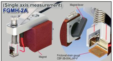
The FGMH-2A is a strain checker especially designed for measurement on a small area such as the vicinity of a welded part. It can be easily attached to and detached from measurement object by the operation of magnet lever. In addition, a lever is provided on the upper part to slightly lift the frictional strain gauge from the measurement surface by pushing the lever downward. It enables easy adjustment of the direction of the strain gauge.
