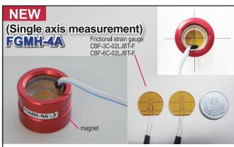
The FGMH-4A is a new, smaller and lighter Frictional Strain Checker that is an evolution of the FGMH-1B.
