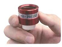
When bonding a strain gauge to the measurement object, it is necessary to keep pressing the strain gauge until the adhesive hardens. PRESSEE is a pressing jig capable of not only pressurizing (PRESS) the strain gauge but also checking the adhesion status from the clear pressing part with eyes (SEE).
