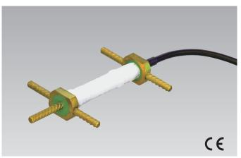
The KM-HAS transducers are embedded into asphalt for measurement of internal strain. The transducers have reinforcing bar flanges at its both ends for good fixation to asphalt pavement materials, and provide for fully waterproof construction. The operating temperature range is -20 to +180°C.
