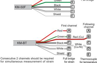
Stranded cables of Red, Green, Black, White and shield to the first channel for strain measurement. Thermocouple of single core Red and White should be connected directly to the following channel for temperature measurement
