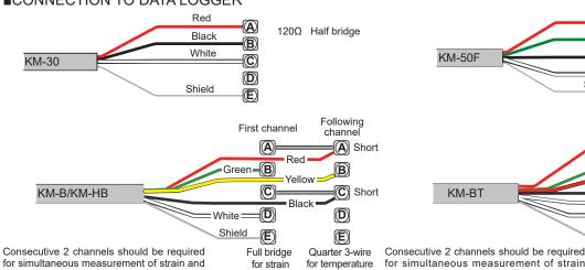
Straded cables of Green, White and shield are connected to the first channel. Remaining cables of Red, Yellow and Black should be connected directly to the following channel for temperature measurement, making short-circuit between A-A and C-C with copper wire for strain measurement.
