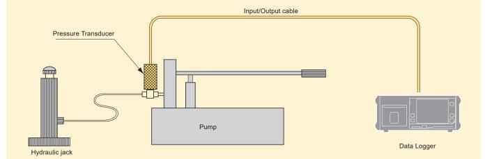
Method used to calculate the conversion coefficient when measuring hydraulic jack load (kN or MN) with a pressure transducer
