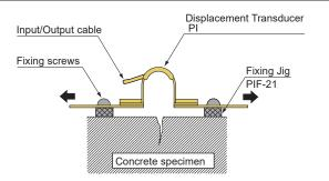
This configuration is used to measure opening displacement due to cracks propagating in concrete.
