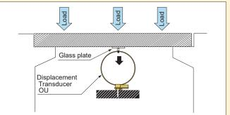
This configuration is used to measure bend with a load applied to a bridge girder.
