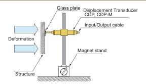
This configuration is used to measure structural deformation and movement.
