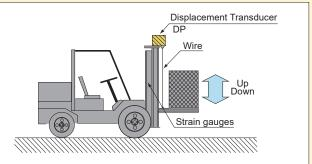
This configuration is used to measure displacement and bending strains in fork-lift truck onboard measurement.
